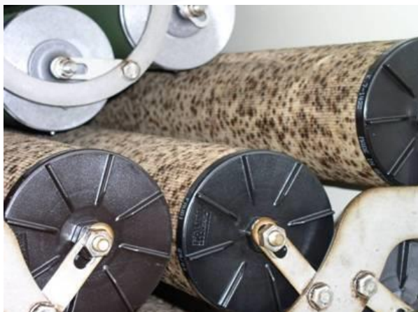
Leopard spotting / fungal growth on Filter Water Separator elements (EI 1581)
