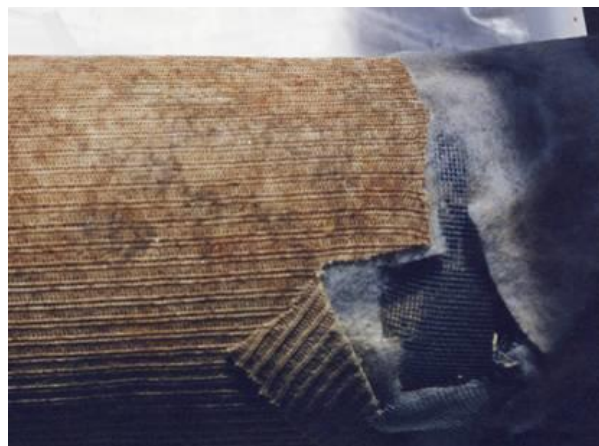
Leopard spotting / fungal growth on Filter Water Separator elements (EI 1581)
