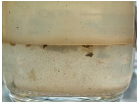
Emulsification at fuel water interface - Microscopic water droplets become suspended in fuel
